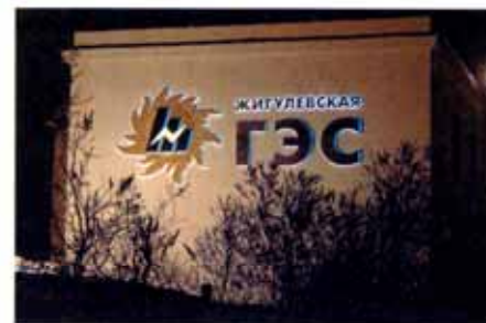
The solar "energy emblem," which sits 42 ft. high, comprises steel tubing, a Dibond® base layer and stainless-steel cladding. Double-halo blue neon and exposed, yellow neon illuminate the emblem and channel letters. The tubes incorporate argon and K4 (a neon and argon mix), which endures cold climates well.
